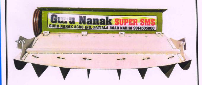
GURU NANAK SUPER SMS, FITTED ON MALKIT 997, SELF- PROPELLED COMBINE HARVESTER
